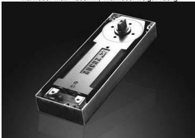
CASA ZC 302 Double Action Floor Spring Max..door width 1200mm, max..door weigth 120kg
