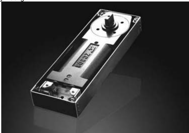
CASA ZC 302 Double Action Floor Spring Max..door width 1200mm, max..door weight 120kg
